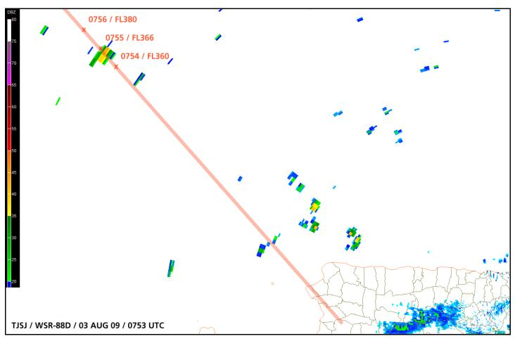
**Figure 6. San Juan PR WSR-88D weather radar** for 3 Aug 2009 at 0753 UTC with flight track superimposed. This showed fairly conclusive evidence that the flight passed through a convective cloud. The radar reflectivity here shows 43 dBZ being returned in a volume between FL220 and FL380. The echo was also detectable at the 1.4 deg elevation, encompassing a bin between FL 360 and FL530. Variations in the refractive index may add further uncertainty to estimated heights.
