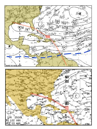
**Figure 2. NCEP surface chart** for 3 Aug 2009 at 0600Z showing much of the region under the influence of the Bermuda High. Solid isopleths indicate stream function, which roughly parallel the wind direction.
