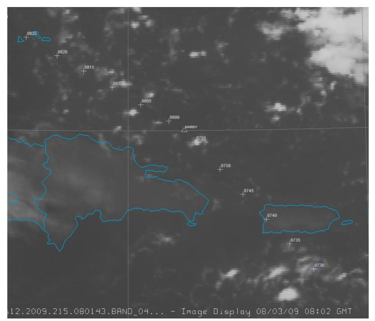
**Figure 5. GOES-12 infrared satellite imagery** for 3 Aug 2009 at 0802Z, with the ASDI flight track superimposed at 5-minute intervals. This indicates that the flight skirted a convective field south of Puerto Rico. This area was probably enough to put the flight crew on guard. The plane then penetrated a cumulonimbus cloud at 0755 UTC north of the Dominican Republic. Cell movement was westward at about 10 kt.
